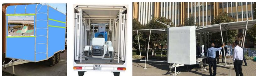
8-rasm. “Quyosh shamol” mobil elektr stansiyasini transport va ishchi xolati
