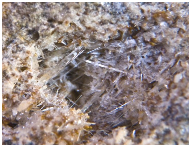
Vollastonitning mikroignasimon tuzilishi (1700 marta kattalashtirib olingan).
