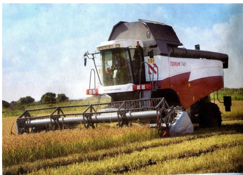
1.34-rasm. TORUM-740 rusumidagi g'alla-don ekinlarini yig'ish kombayini
