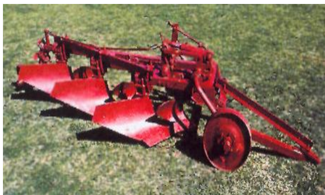
1.12-rasm. PYA-3-30 ikki qavatli tirkamali plug
