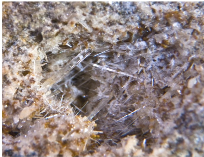
Microneedle structure of wollastonite (magnified 1700 times).
