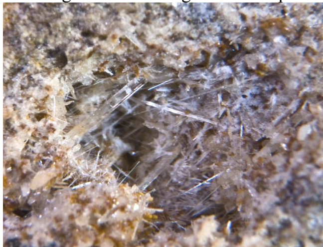
Vollastonitning mikroignasimon tuzilishi (1700 marta kattalashtirib olingan).
