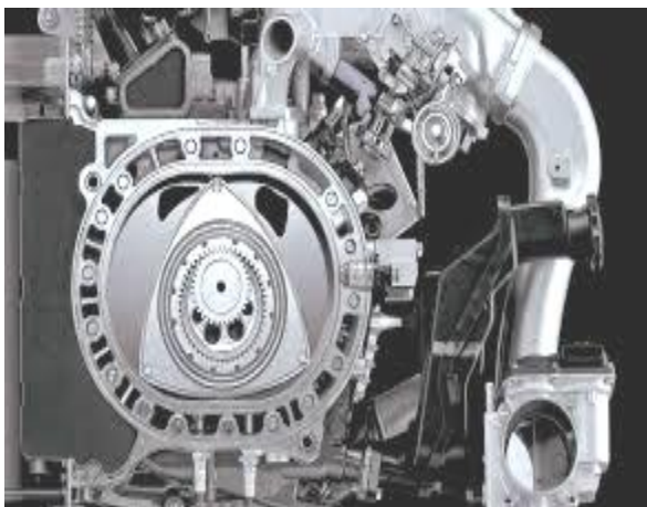
3.8-rasm. Rotor-porshenli dvigatelning ishlash sxemasi:
