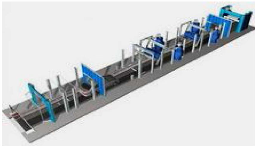
4-rasm. Avtomobillarni yuvish konveyeri shakli (konveyerning harakatlanish tezligi 3...4 m/min).
