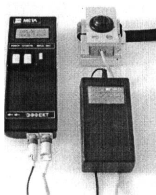
Tormoz tizimining samaradorligini aniqlovchi EFFEKT-02 jihozi
