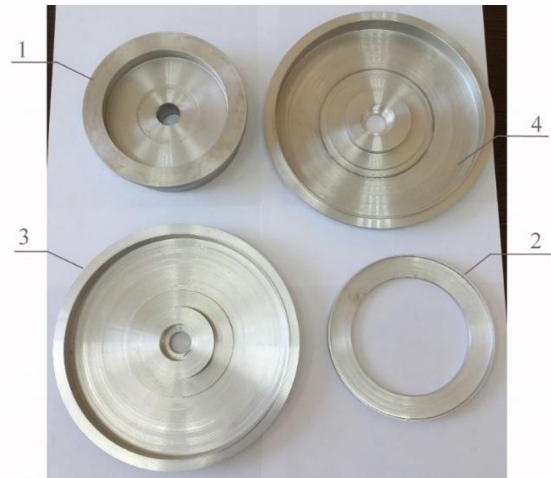
Fig. 3. Produced elements of the motor-wheel housing: 1 – stator, 2 – clamping ring, 3 – protective cover, 4 – brake cover
