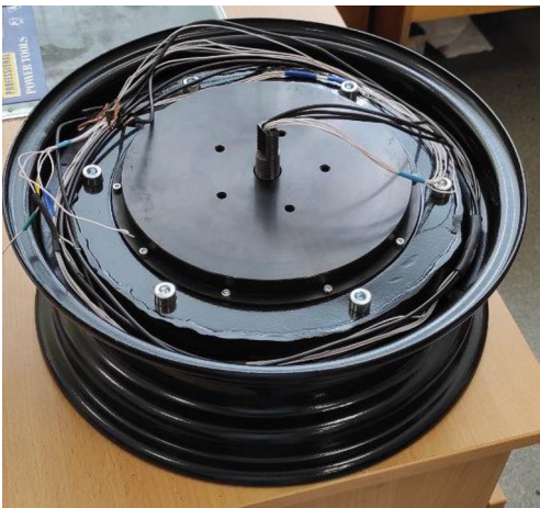
Fig. 6. Appearance of an experimental sample of a motor-wheel
