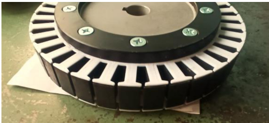
Fig. 3. Produced elements of the motor-wheel housing: 1 – stator, 2 – clamping ring, 3 – protective cover, 4 – brake cover
