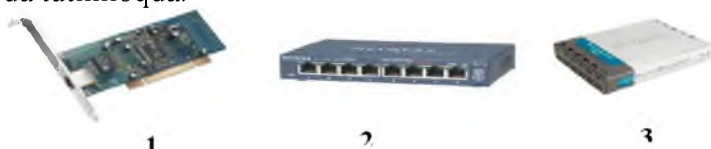
10.1-rasm. Tarmoq qurilmalari (1-tarmoq adapter, 2-komuttator (svitsh), 3-marShuritizator (router)).
