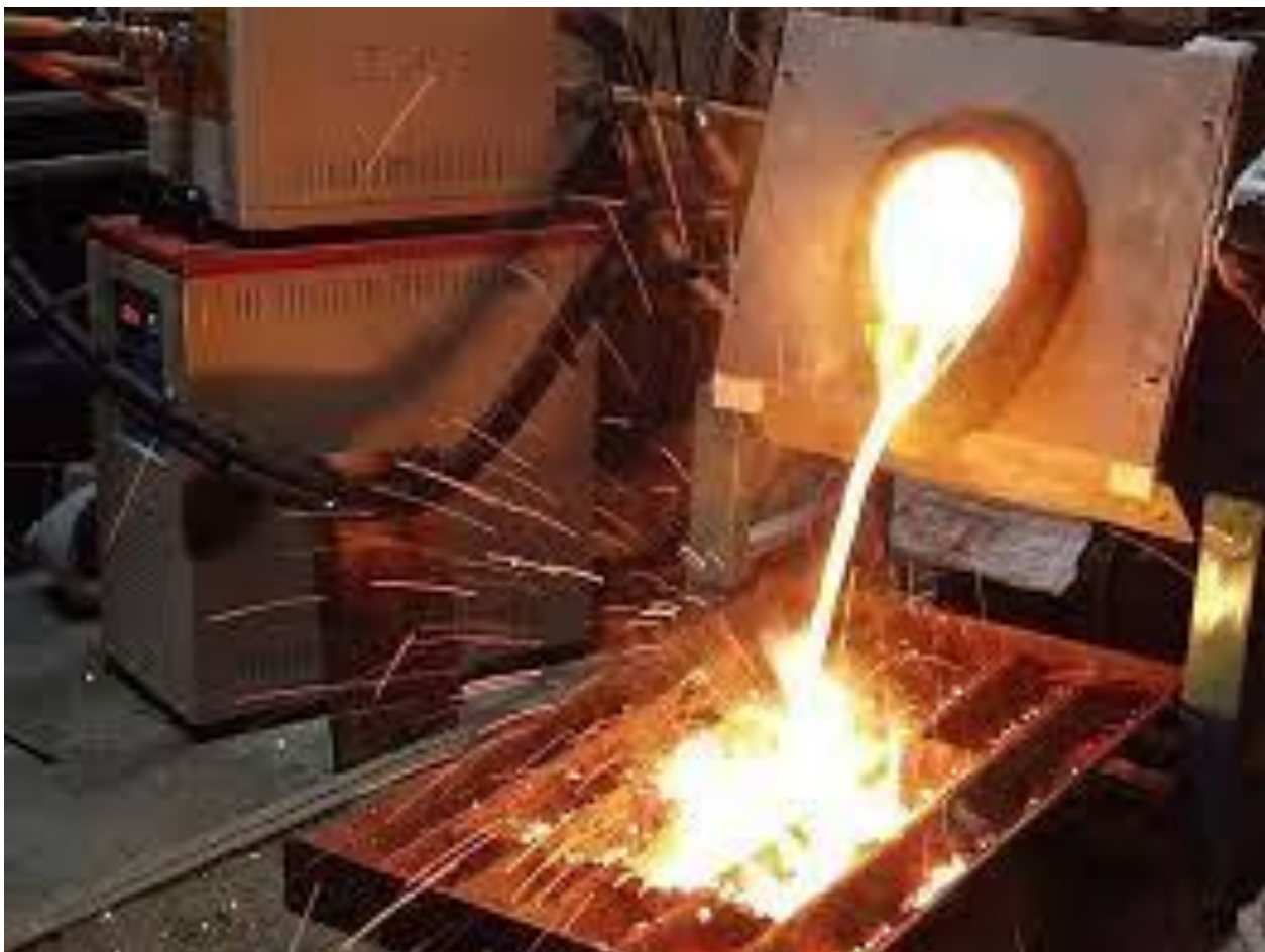
3 – rasm. Induksion pechidan qilopga quyish jarayoni
