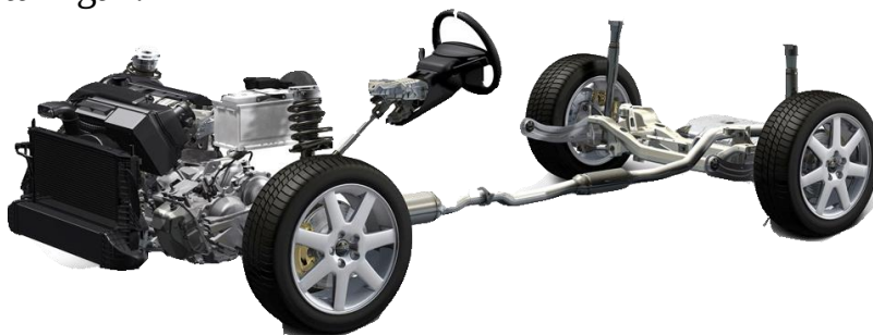
2.2-rasm. Yengil avtomobil yurish qismi.
