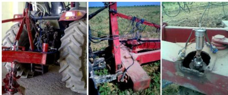
8-rasm. Tenzometrik plugning ayrim ko‘rinishlari
