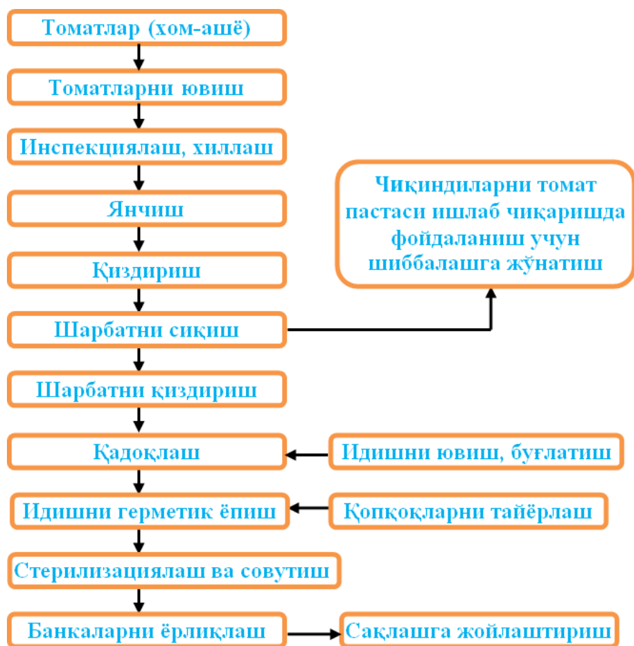
1-rasm: b) Tomat sharbati ishlab chiqarishning texnologik sxemasi
