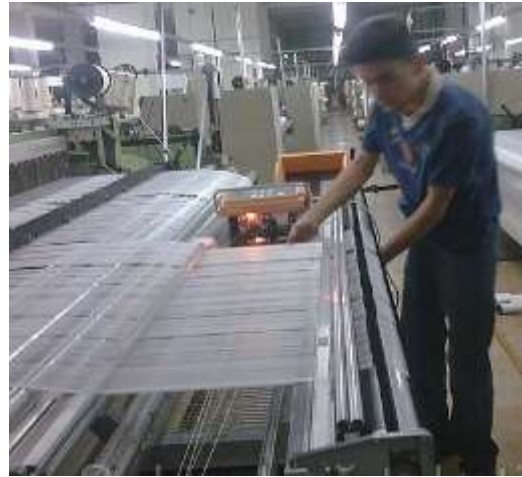
4.8-rasm. Bog‘lash mashinasi va aravachasining ko‘rinishi
