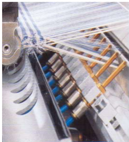
5.18-rasm. Zultser Ryuti L5100 pnevmatik to'quv dastgohining estafetali purkagichlari
