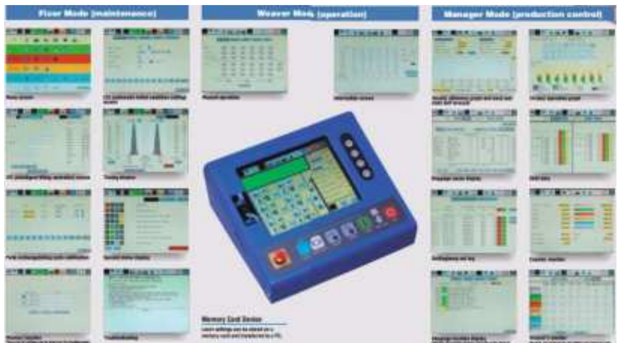
5.4-rasm. Toyota to'quv dastgoxining texnologik omillarni boshqaruv - nazorat monitori
