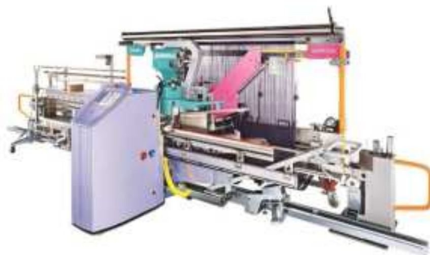
4.5-rasm. Avtomat ip o‘tkazish mashinasi (Staubli).
