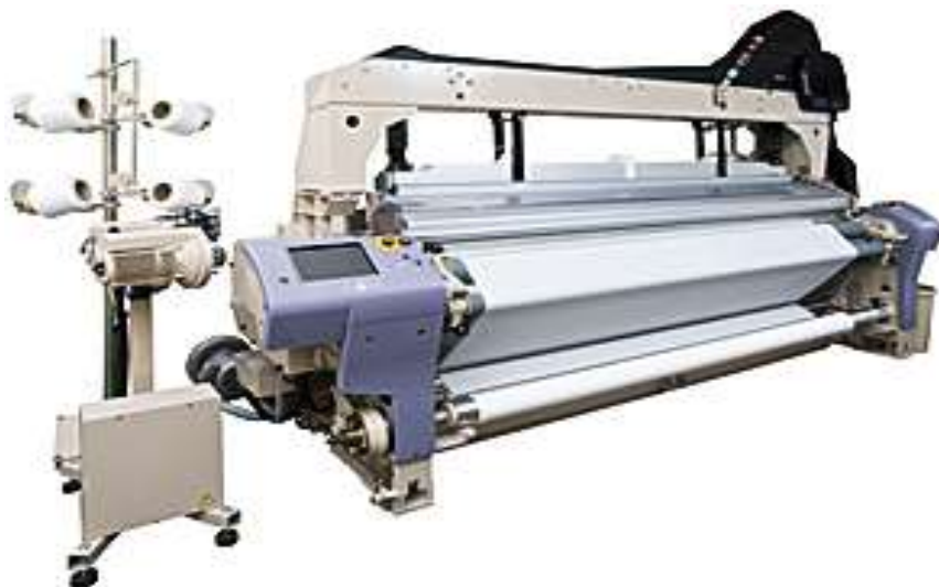
5.30-rasm. Tsudakoma “ZW8100” gidravlik to'quv dastgohi
