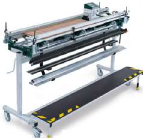
4.8-rasm. Bog‘lash mashinasi va aravachasining ko‘rinishi
