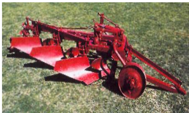
1.12-rasm. PYA-3-30 ikki qavatli tirkamali plug
