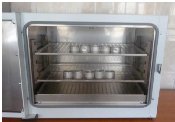
8.3.-rasm. Olingan tuproq namunalarini termostatda (quritish shkafi) quritish
