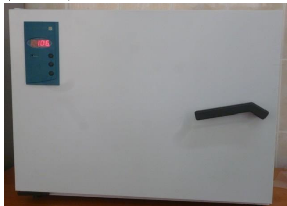
8.3.-rasm. Olingan tuproq namunalarini termostatda (quritish shkafi) quritish
