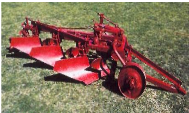
1.12-rasm. PYA-3-30 ikki qavatli tirkamali plug
