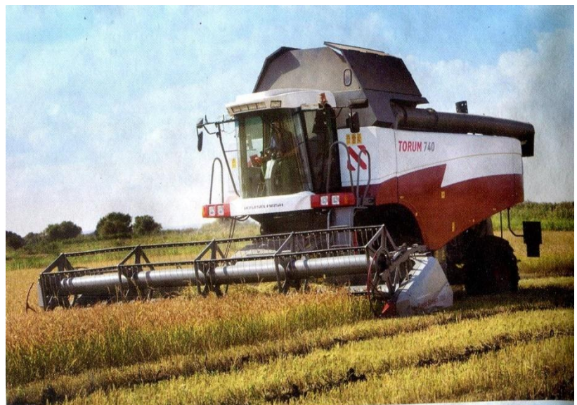
1.34-rasm. TORUM-740 rusumidagi g'alla-don ekinlarini yig'ish kombayini
