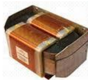
9.10-rasm. Lak ham izolyator, ham kley vazifasini bajaradi
