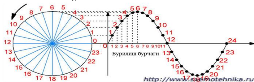
4.2-rasm. Sinusoidal kuchlanishning hosil bo'lishi.
