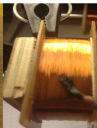
9.10-rasm. Lak ham izolyator, ham kley vazifasini bajaradi
