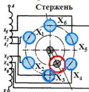
1.42-rasm. Uch fazali transformator chulg'ami rostlovchi ulanishlarining sxemalari
