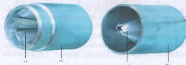
5-rasm. Takomillashtirilgan prujinali kern ushlagich: 1-prujinali kern ushlagich; 2-korpus.
