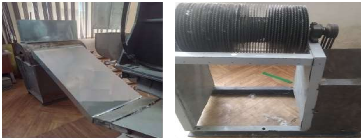
4-rasm. 1VPU rusumli tola tozalagichning laboratoriya nusxasi
