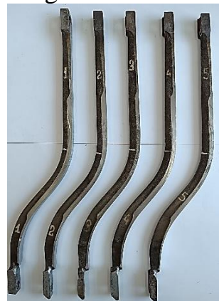
14-rasm. Chidamlilikni sinash uchun jin nazorat kolosniklari
