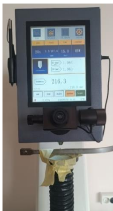
9-rasm. HRS-300E qattqlik o‘lovchi priborning o‘lchov-registratsiya blogi
