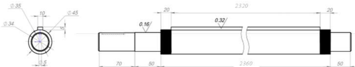
10-rasm. Tezlatkich-surgich valining ishchi chizmasi
