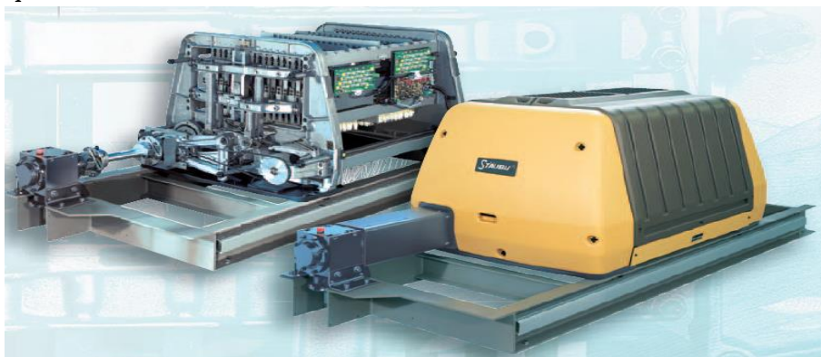
7.12-rasm Staubli firmasining SX 870 jakkard mashinasi
