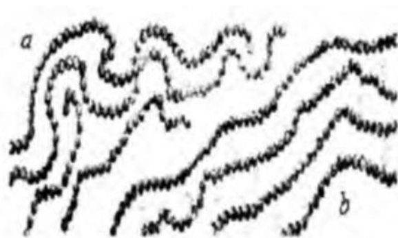
2-rasm. Kauchukning (a) va rezinannig (b) tuzilishi.
