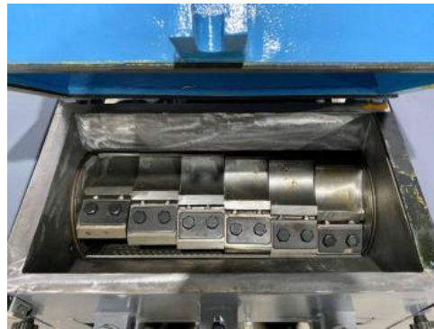
2-rasm. "Model - EC600": Quvvat iste'moli: 15 kVt. Kuchlanish: 380 V.
