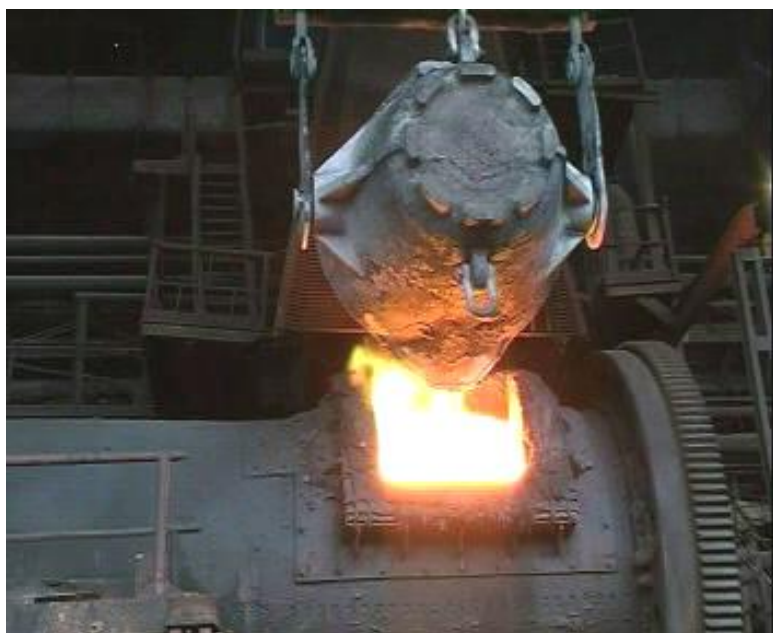
4.16-rasm. OTMK Mis eritish zavodida homaki misni olovli tozalash bosqichi
