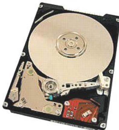
7.2-rasm. Hitachi Travelstar vinchesteri
