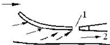
3.8-rasm. Egri suv ushlagich shpora. 1 - suv tashlagich, 2 - kanal.
