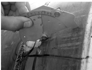
4.3.1-rasm. Payvand chokining qirqilish chuqurligini vizual nazorat qilish.
