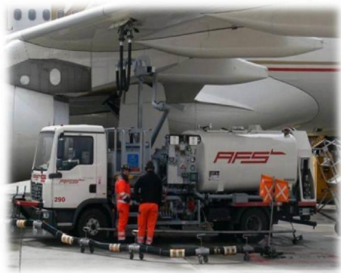
2.21-rasm. Hidrantli yoqilg'i quyish mashinasi "Superflow PHD 7.000"
