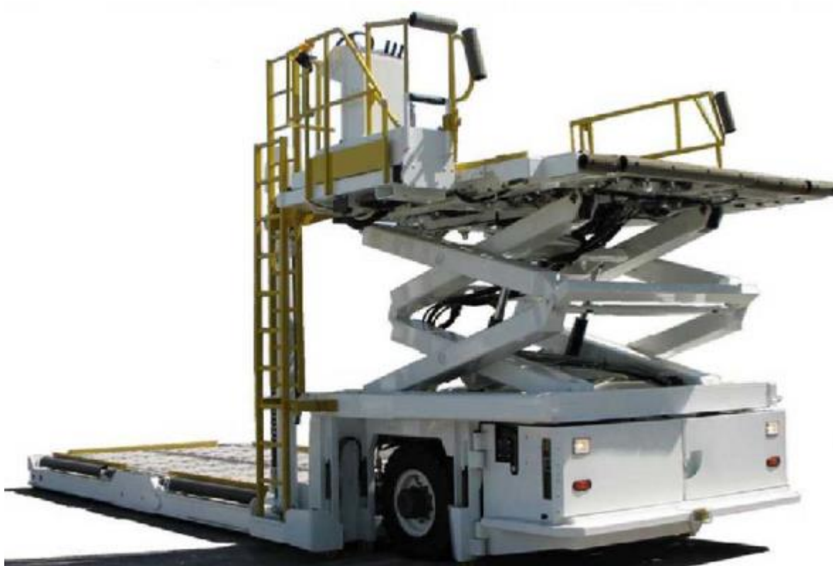
2.2-rasm. Yuk yuklovchi “FMC Commander-30 I Universal”
