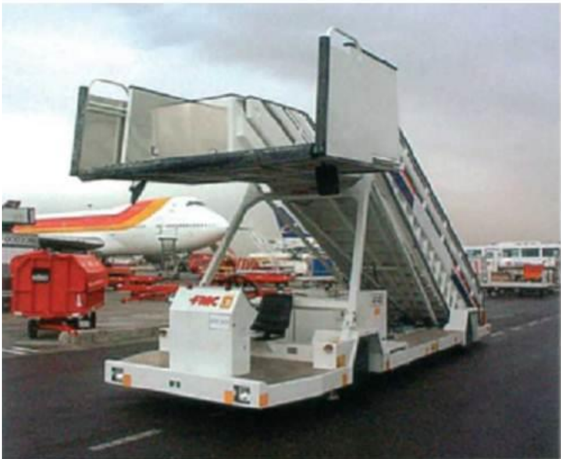
1.11-rasm. Yo'lovchilar trapi "SMARTSTEP-2"
