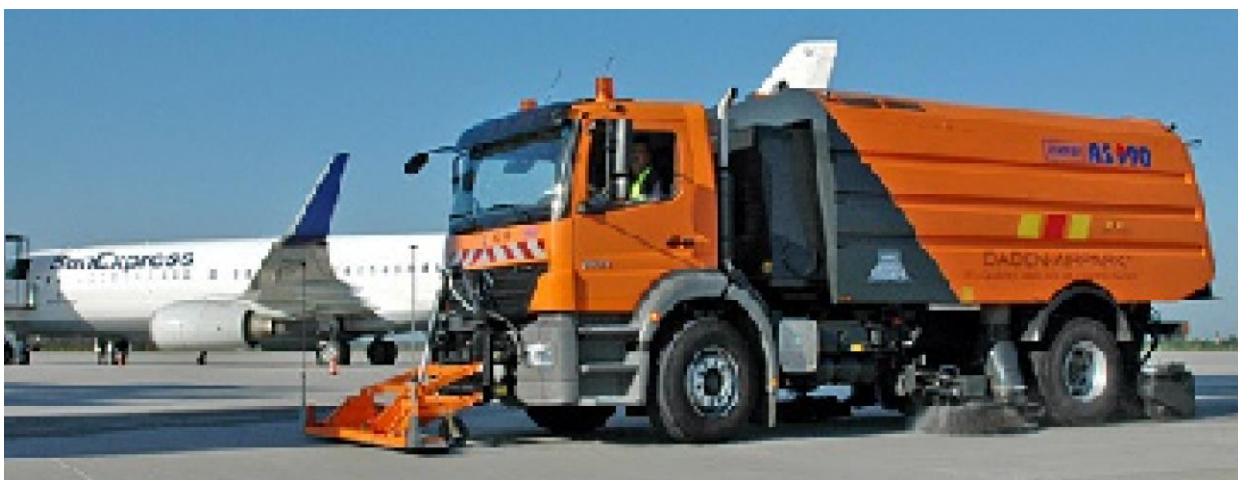
3.16-rasm. Aerodrom hududini tozalovchi mashinasi “SCHMIDT AS 990”
