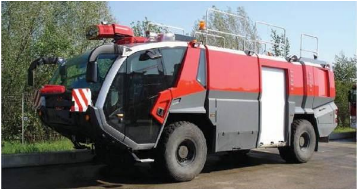
2.9-rasm. Aeroportning o't o'chirish mashinasi "PANTHER 4x4-3.0_CA6"
