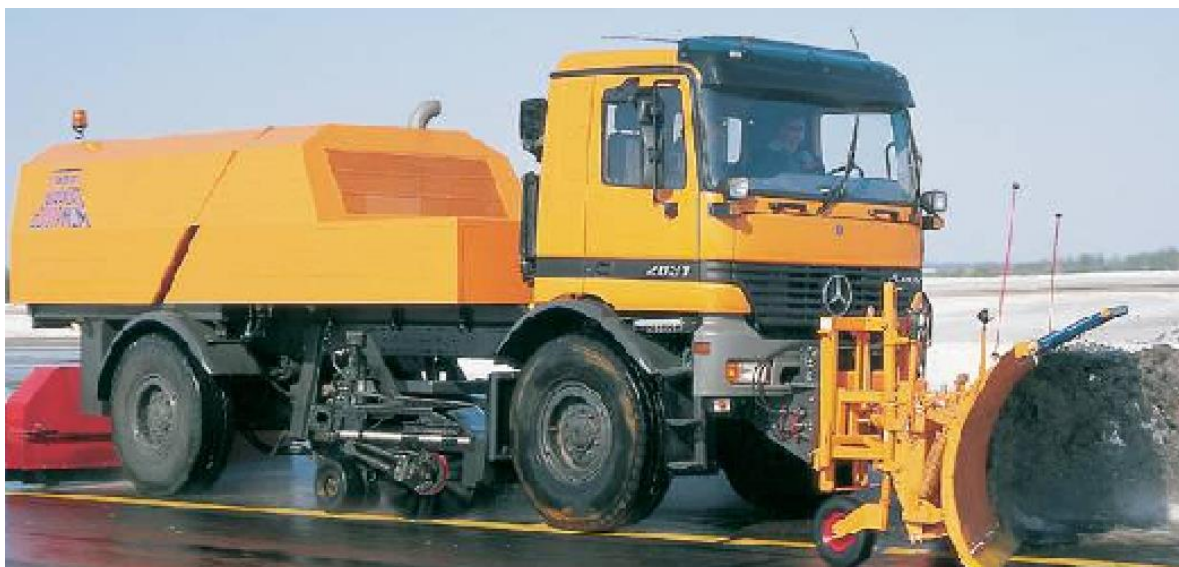
3.6-rasm. Qor supirish mashinasi “Compact Jet Sweeper SJS 914 Super II”
