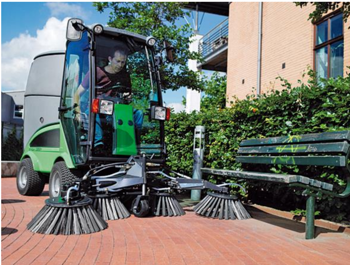
3.17-rasm. Aerovokzal hududini tozalovchi mashinasi “EGHOLM”
