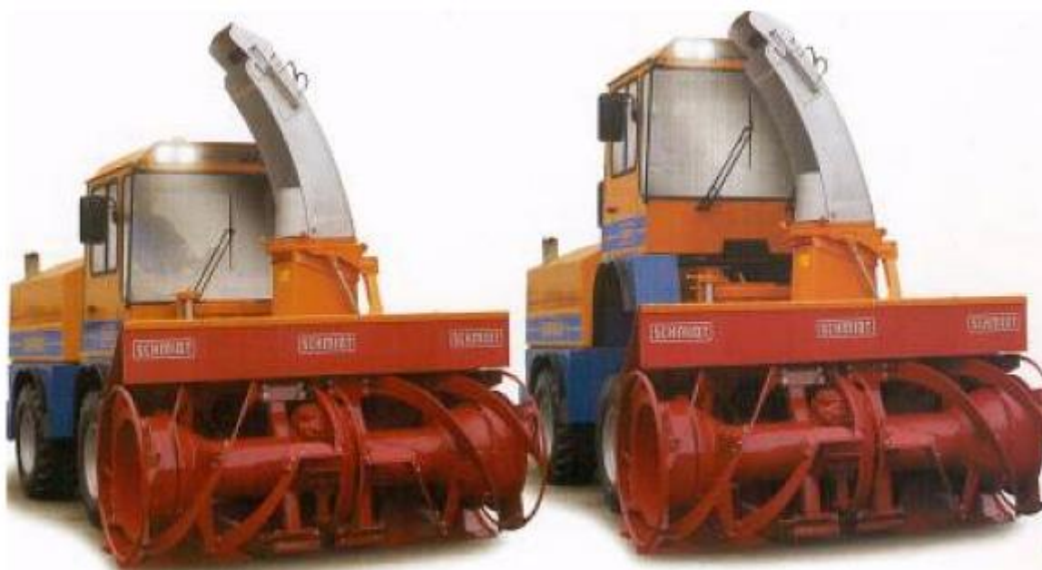
3.10-rasm. Rotorli qor tozalash mashinasi “SUPRA 4001”
