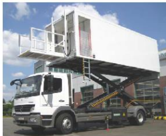
1.5-rasm. Oshxona xizmati avtolifti “STEWART LV 28.61”
