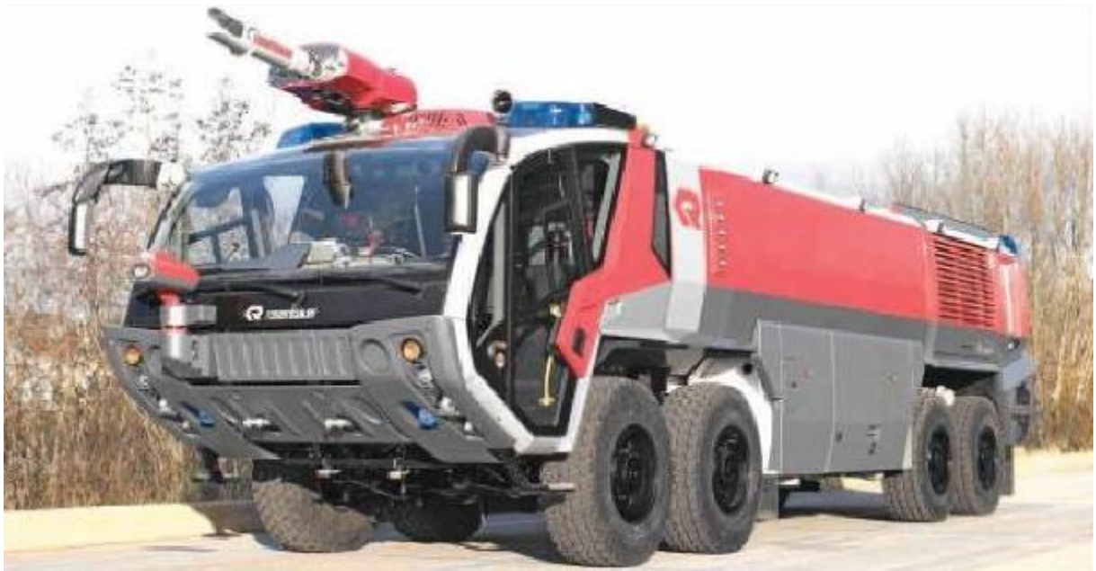
2.11-rasm. Aeroportning o't o'chirish mashinasi "PANTHER 8x8_CA7"
