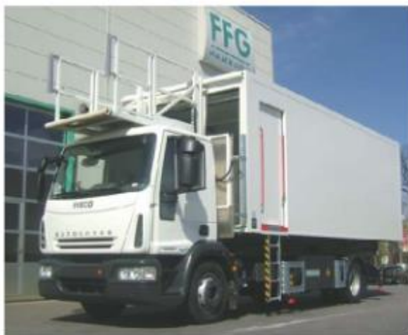
1.5-rasm. Oshxona xizmati avtolifti “STEWART LV 28.61”
