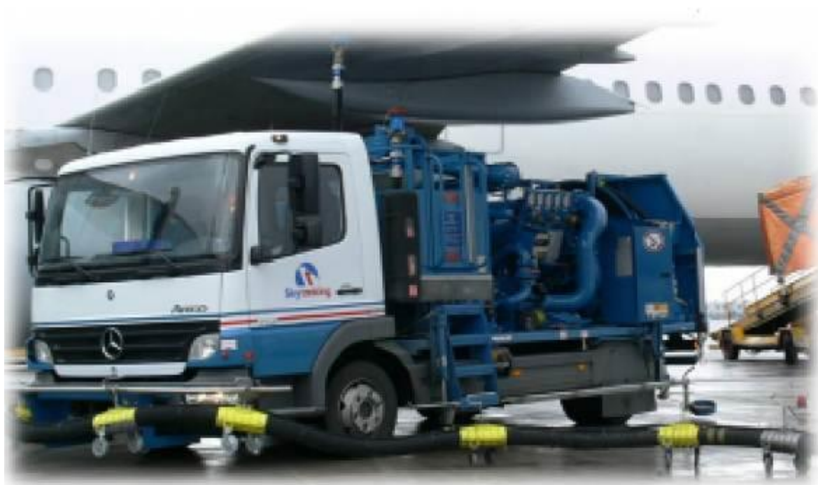
2.22-rasm. Gidrantli yoqilg'i quyish mashinasi "Gidrant-dispenser"
