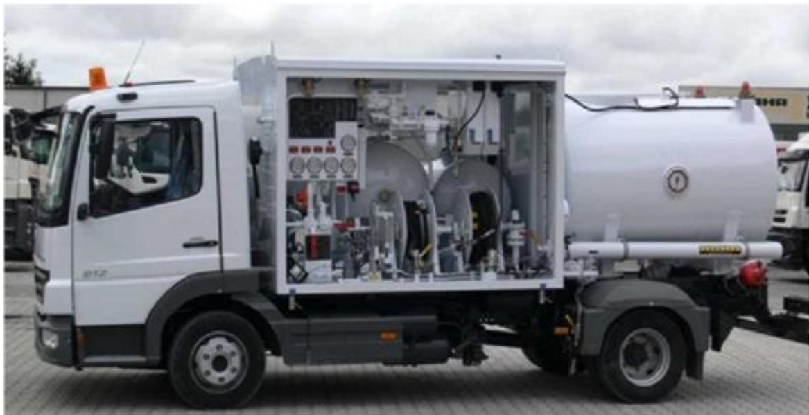
2.6-rasm. Havo kemasini yuvish mashinasi "Mercedes Benz Vario614 D/4x2"
