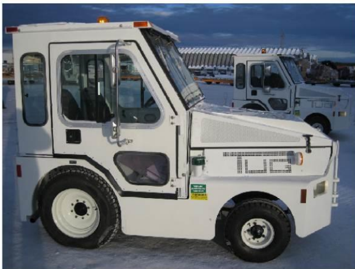
2.24-rasm. Yuk aravachalarini shatakka oluvchi mashinasi “M1A”
