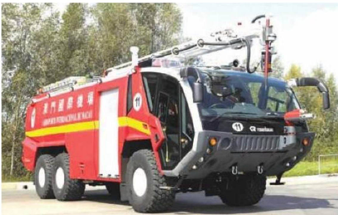
2.10-rasm. Aeroportning o't o'chirish mashinasi "PANTHER 6x6_CA5-HRET"
