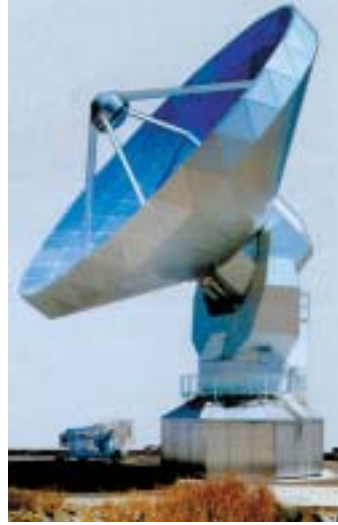
57- rasm. Parabolik antennali radioteleskop.
