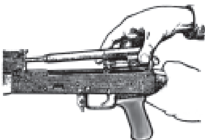
100-rasm. Zatvor ramasini zatvor bilan birga ajratish.
