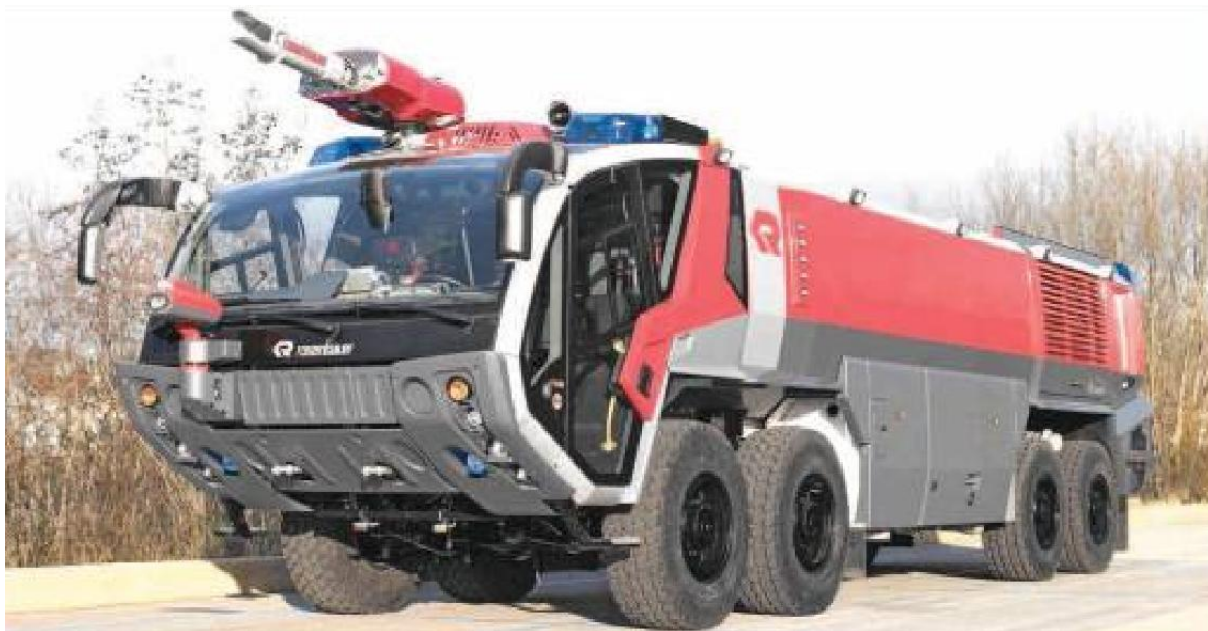
2.11-rasm. Aeroportning o't o'chirish mashinasi "PANTHER 8x8_CA7"
