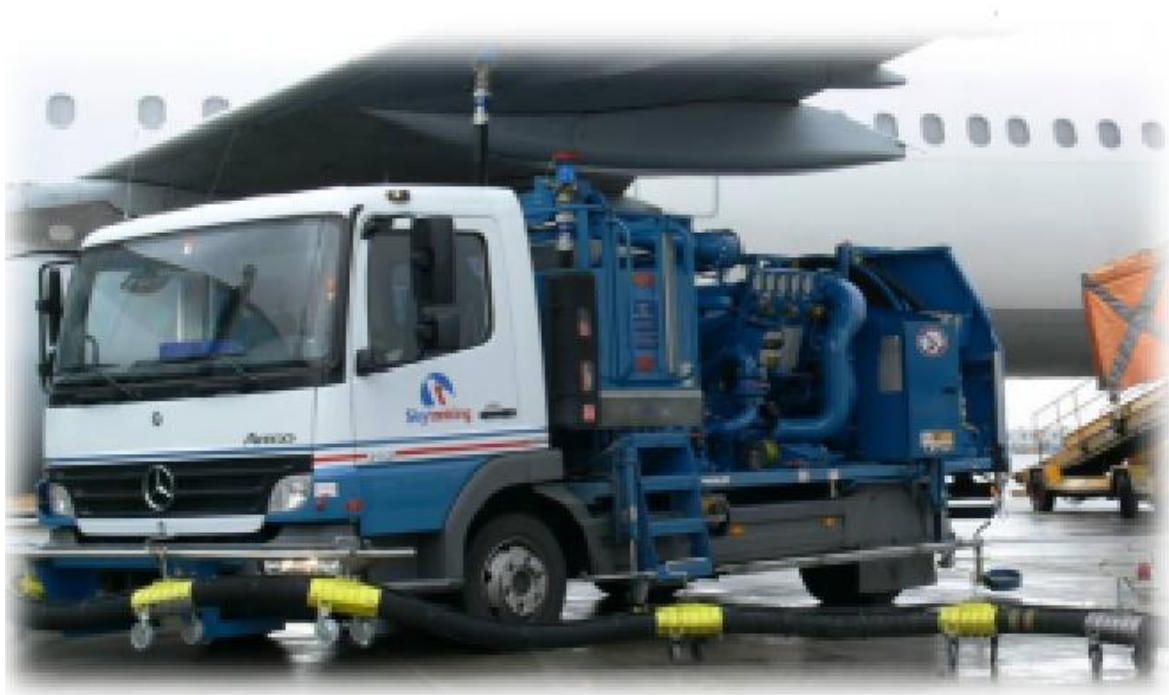
2.22-rasm. Gidrantli yoqilg'i quyish mashinasi "Gidrant-dispenser"
