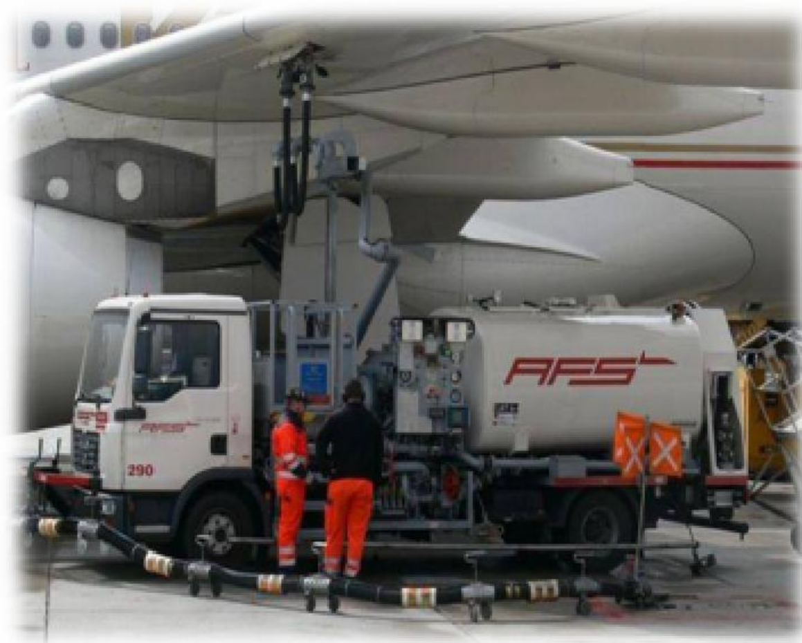
2.21-rasm. Gidrantli yoqilg'i quyish mashinasi "Superflow PHD 7.000"
