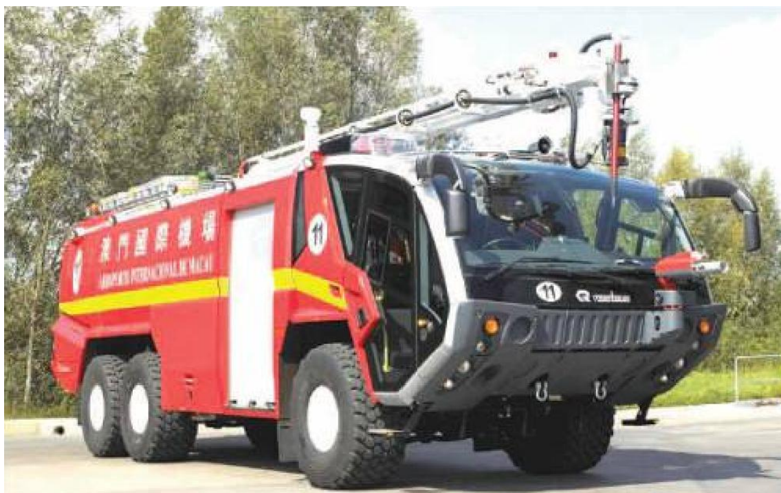
2.10-rasm. Aeroportning o't o'chirish mashinasi "PANTHER 6x6_CA5-HRET"
