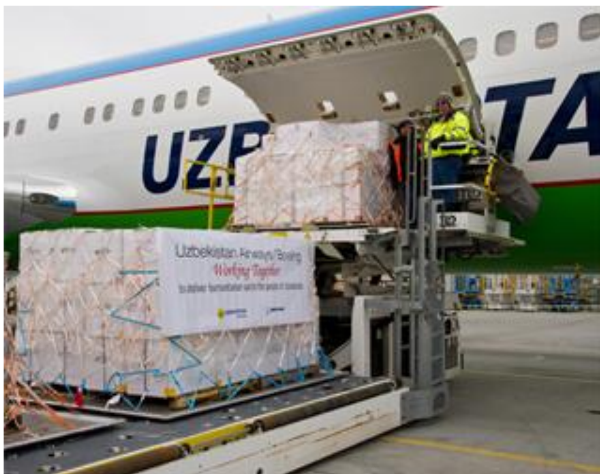
2.3-rasm. Yuk yuklovchi “Commander”
