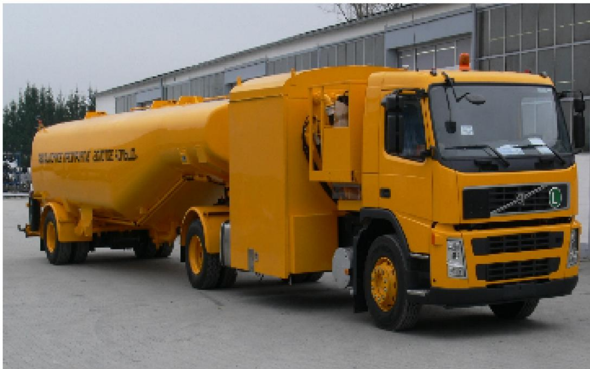
2.20-rasm. Havo kemasiga yoqilg'i quyish mashinasi "SCANIA"
