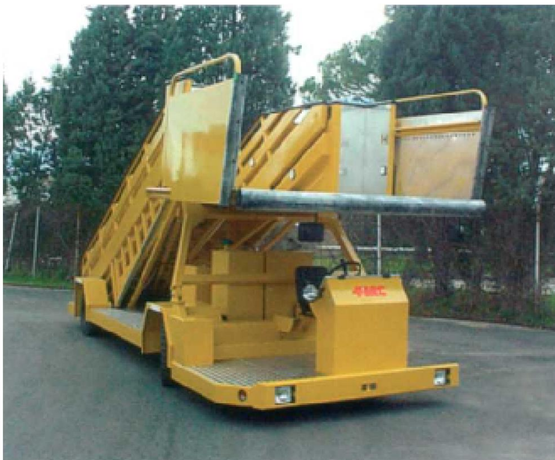
1.12-rasm. Yo'lovchilar trapi "NBS-2"
