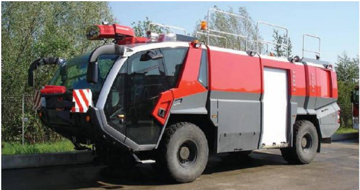
2.9-rasm. Aeroportning o't o'chirish mashinasi "PANTHER 4x4-3.0_CA6"
