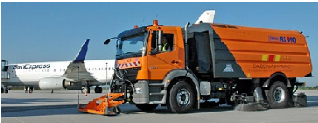
3.16-rasm. Aerodrom hududini tozalovchi mashinasi “SCHMIDT AS 990”
