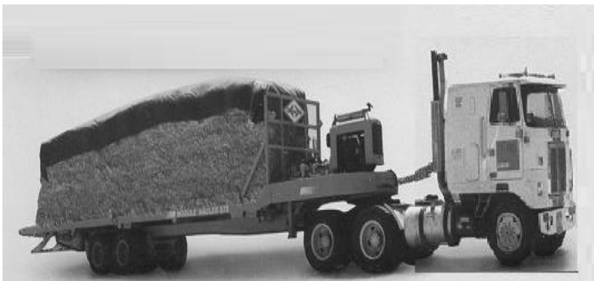
11.3- rasm. Paxta modulini tashuvchi treyler
