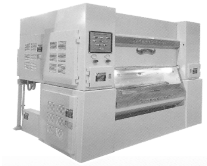
11.18-rasm. “Fenniks Rotobar” valikli jinining tashqi ko’rinishi. 1.Tozalagich-ta’minlagich; 2.Valikli jin;
