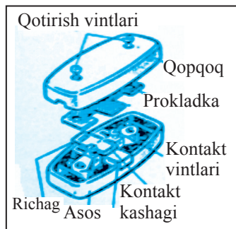
75-rasm. Osma vkluchatel tuzilishi.
