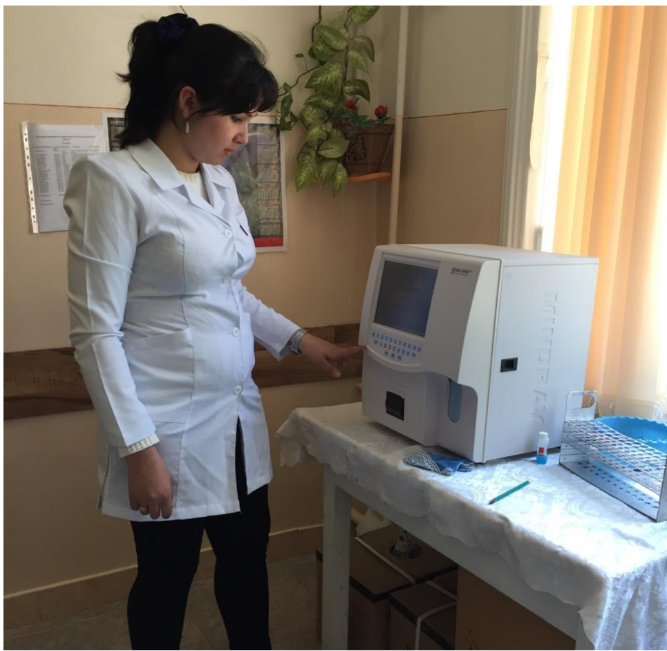
2.1- rasm. Mibi Screen- biokimyoviy va immunoturbodemetrik usullarni bajaradi
