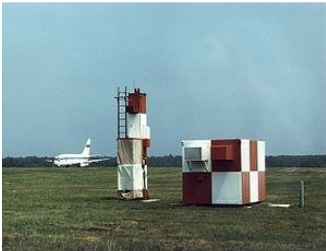
The NASA 737 research aircraft on the Wallops runway in 1987 with the Microwave Landing System equipment in the foreground.
