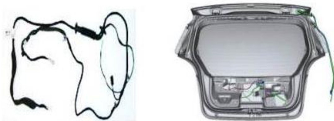
6-rasm. Wiring Harness-TAIL GATE- avtomobil orqa yukxona elektr tizimlari jguti;
