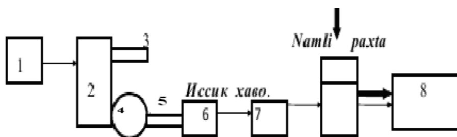
5-rasm. Nam chigitli paxtani quritish texnologik jarayoni.
