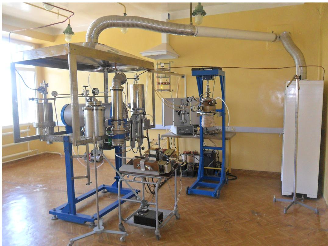
**Fig.1.4. General view of the experimental setup for the implementation of the process of synthesis of monosilane**
