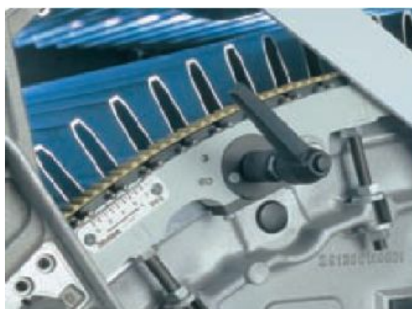
29-su'wret. Shlyapkalardi tuwrilawshi precizion PFS sistemasi
