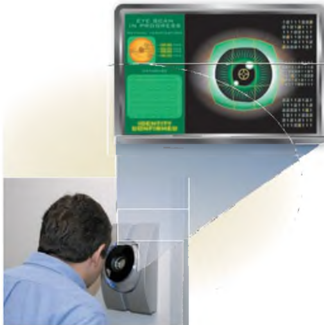
Figure 5-11 An iris recognition system.
