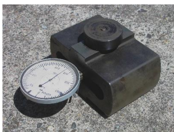
400 kN ǵa shekemgi kúshlerdi ólshew ushın arnalǵan dinamometr.
