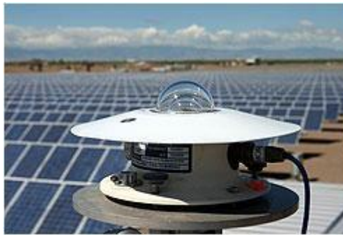
a) Thermopile-type pyranometer
