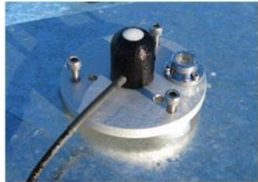
b) Photovoltaic detector-type pyranometer.
