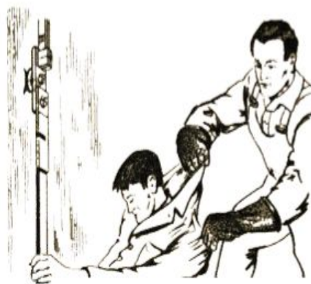
4.1-rasm. Elektr toki ta'siridan ajratib olish
