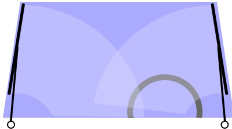
12-rasm. Qarama-qarshi faqat oyna tozalagichning yuritma elementlari old oynaning ikki chetida (SEAT Altea, SEAT León Mk2, SEAT Toledo Mk3 kabi avtomobillarda).
