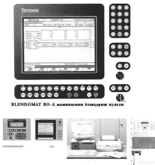
21-rasm. Truchler firmasining VLENDCOMMANDER nazorat qilish va boshqarish tizimi
