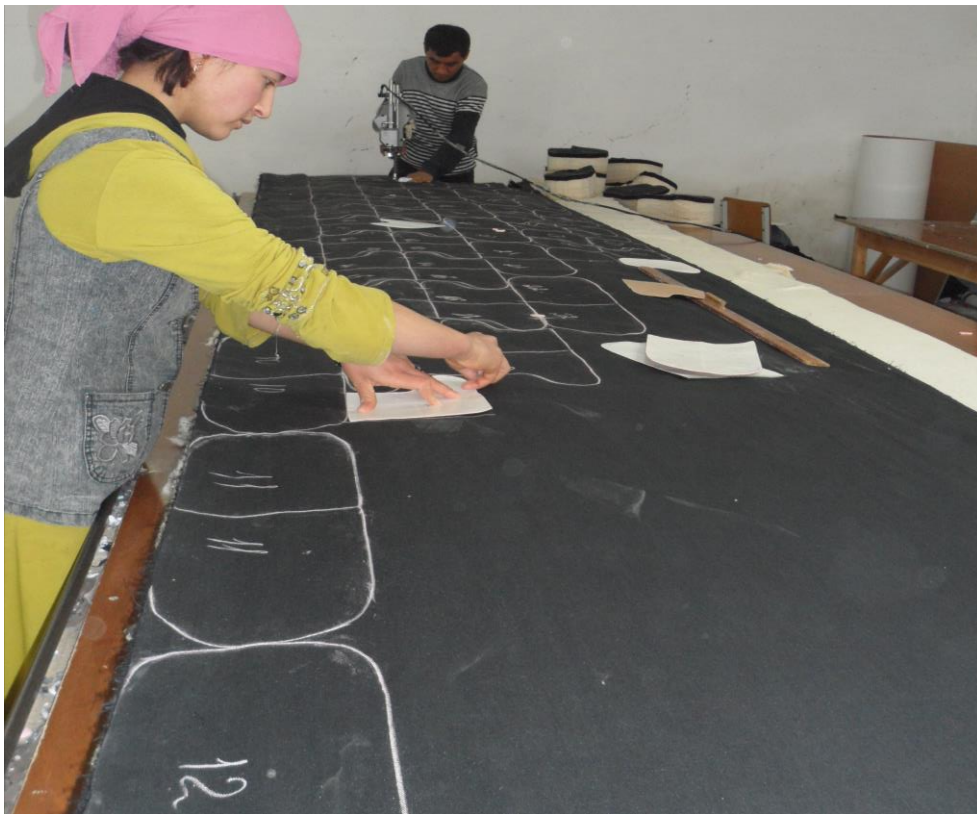
9-rasm. Bichish jarayonida yuuyum detallarni bo'rlab chiqish
