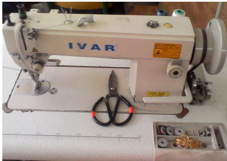
3.8-rasm. To`gri baxyaqator yuritib tikuvchi "IVAR" maxsus sumka tikish mashinasining ko`rinishi
