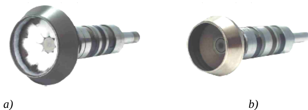
14-rasm. Teshikli (a) va teshiksiz (b) kameralar
