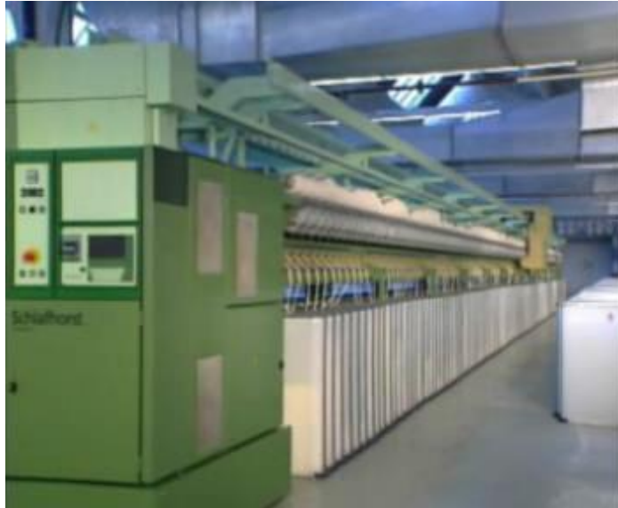
8-rasm. Shlyafxorst firmasining pnevmomexanik yigirish mashinasi
